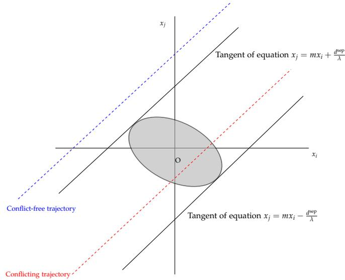
To derive an analytical expression of this condition, the author uses the two tangents of the ellipse that are parallel to the parametric line  $(x_i(t), x_j(t))_{t \geq 0}$ . Their equations are given as follows:
